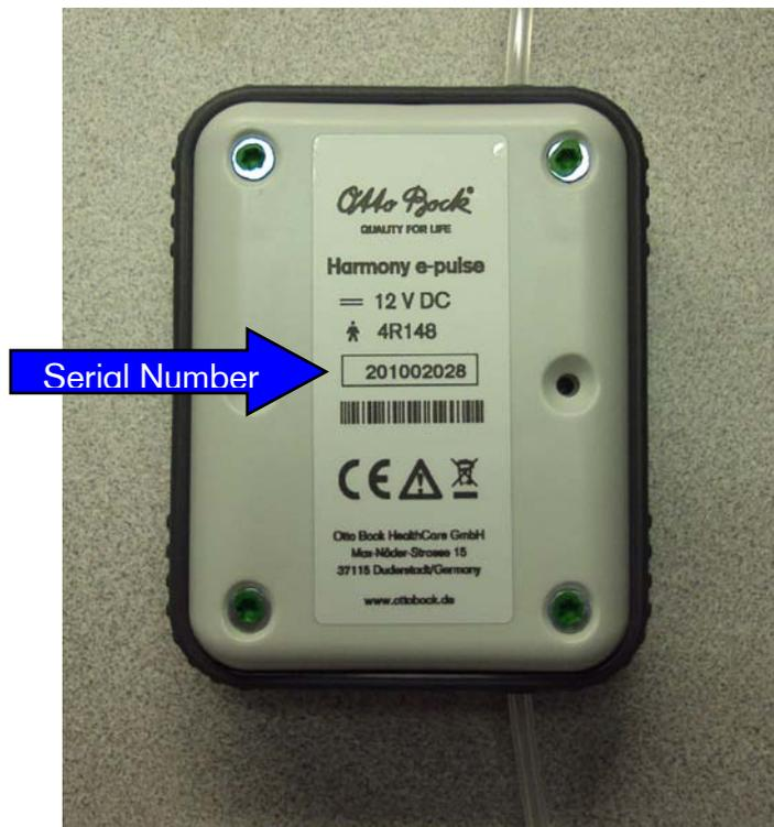
**Or test the pump:** Another way to test for which pump version you have is to turn the pump on and hold the "+" for 3 seconds. The new/upgraded pumps will go into the flush mode in which the pump cycles very fast with a different sounding pitch and lights 1 and 4 are lit.
